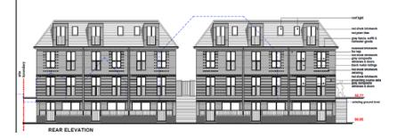
Figure 3 Proposed rear elevation showing lower ground floor
